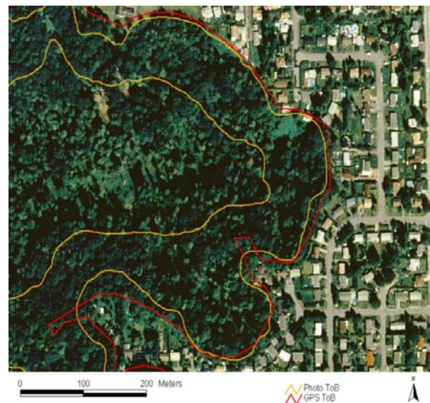
Fig. 3. ToB determined for an area with a clearly defined forest-urban boundary, using photogrammetry versus ground-based GPS surveying.
