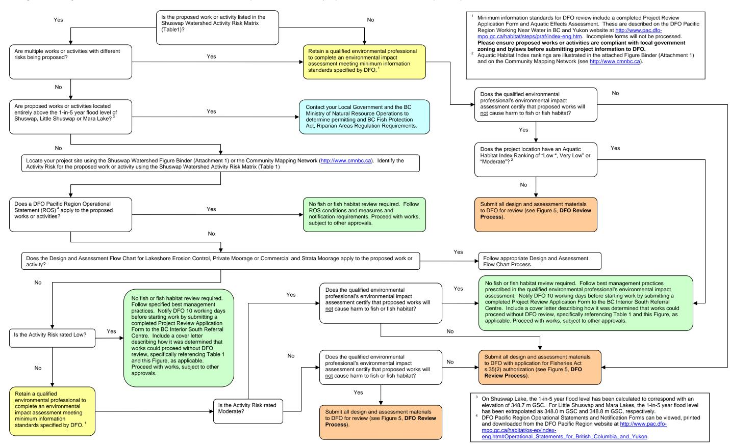
Figure 2 Design and Assessment Flow Chart for Lakeshore Erosion Control on the Shuswap Lake System
